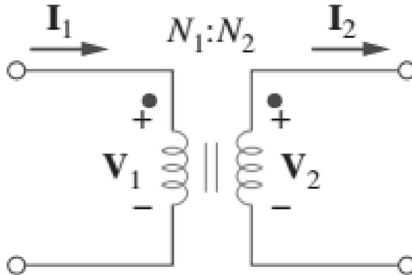
$$\left\{ \begin{array}{l} \frac{V_2}{V_1} = \frac{N_2}{N_1} \\ \frac{I_2}{I_1} = \frac{N_1}{N_2} \end{array} \right.$$
